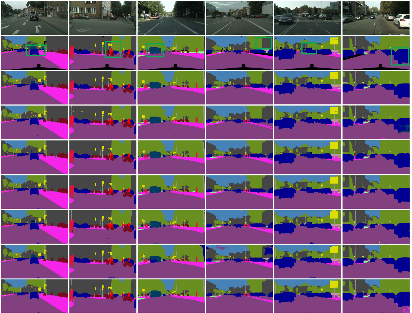
Fig. 6. The comparative results on the Cityscapes val dataset. From top to the bottom are successively the original observed images, ground truths, segmentation results from our MSCFNet, LEDNet [23], DABNet [22], ERFNet [18], EDANet [27], CGNet [47] and ESPNet [36]. (Best viewed in color).
