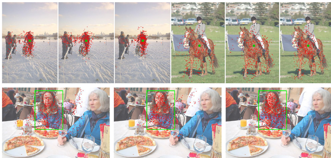
Fig. 5. The visualization of effective sampling locations. Each triplet of images denotes the spatial support of the method using standard, modulated or adaptive modules respectively, with using deformable convolution@conv3-conv5. The images in second row are produced by the methods which use corresponding deformable Rolpooling.
