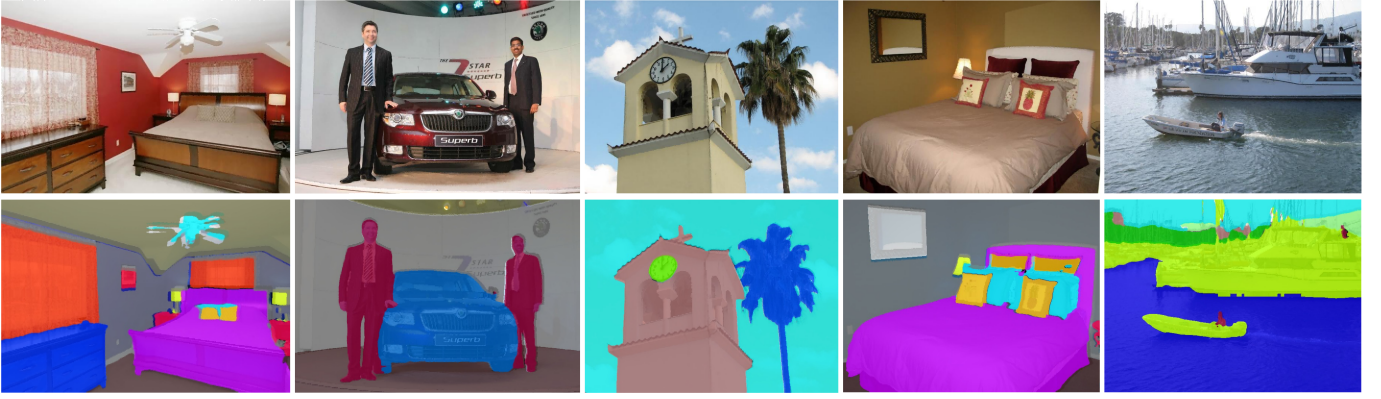
Fig. 6: Qualitative results of semantic segmentation on ADE20K val dataset [77]. Upper: input validation images, Lower: results generated by S2AFormer-S-based Semantic FPN [78].
